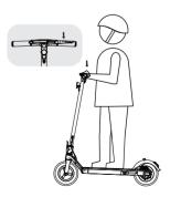
4To slow down the scooter, disengage the accelerator and squeeze the brake handle to engage the e-brake and disc brake
