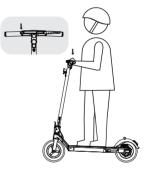
2 The harder you squeeze the acceleration trigger, the faster you will speed up
