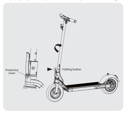
Step 2: Folding down the steering column, Align the locking clasp with the side of the locking hook, then buckle into the locking hook in parallel
