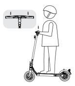
4 To slow down the scooter, disengage the accelerator and squeeze the right brake handle to engage the e-brake and disc brake or squeeze the left brake handle to engage the drum brake
